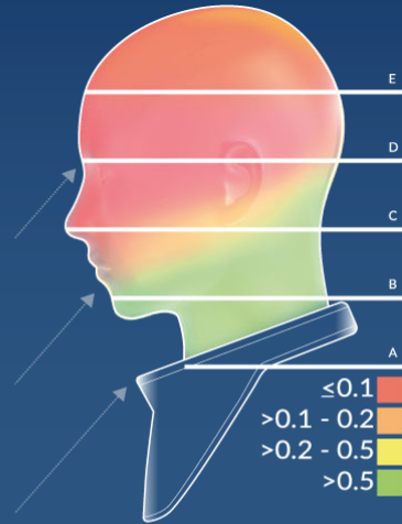
Schematic illustration of the reduction ratios for a standard thyroid collar in phantom slices A, B, C, D, E for the investigated exposure situation.
