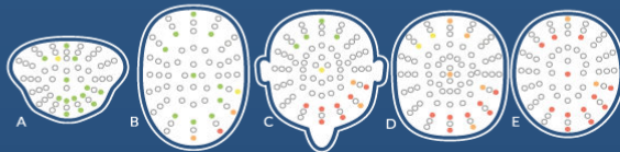
Schematic illustration of the reduction ratios for a standard thyroid collar in phantom slices A, B, C, D, E for the investigated exposure situation.
